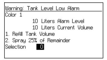
Fig. 16. Tank Level Low Screen (Tank A Shown)
